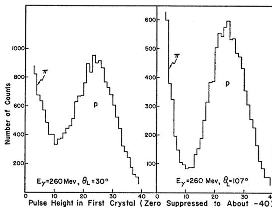
FIG. 2. Differential pulse-height spectra in first crystal for particles of defined residual range. The resolution shown for 107° is typical of that obtained at all other lab. angles except 30°.
