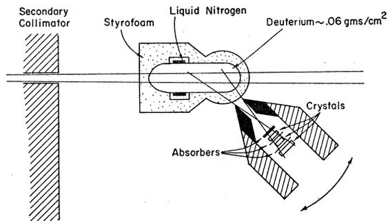
FIG. 1. Diagrammatic view of apparatus with compressed gas target.
