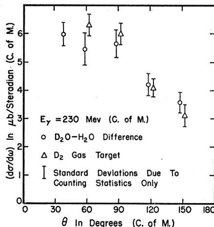
FIG. 5. Differential cross section for photodisintegration at 230 Mev (c.m.).
