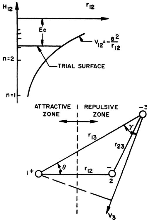
FIG. 1. Schematic diagram showing location of "trial" surface separating "free" and "bound" states of an electron-ion pair and geometry of the three-body collision.
