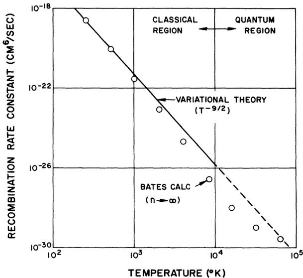
FIG. 2. Comparison of present results with those calculated by Bates for infinite electron density using Gryzinski's classical transition probabilities. Note that the extension of either Bates' or the present results into the quantum mechanical region is of doubtful validity.
